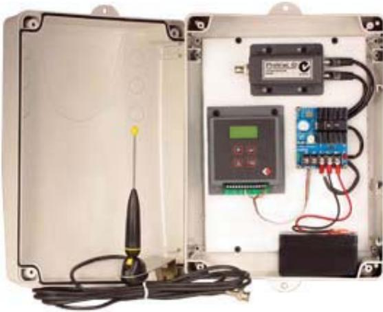
Long Range, Hands-Free Stand Alone RFID Reader System designed to provide fast and secure gate access control at gated communities and commercial facilities for all first responders, including police, fire, rescue and private security vehicles.
